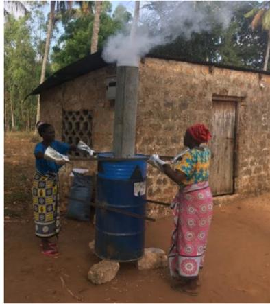
The furnace above was developed with members of BioSmart in conjunction with the University of Exeter Engineering department. It was created to use materials that are readily available in Kadzinuni. The Biochar that is produced is bound with casava paste which creates a briquette. These briquettes can then be sold to the local people. We have four in use in Kadzinuni, and we have plans to build more here and in Zanzibar.
